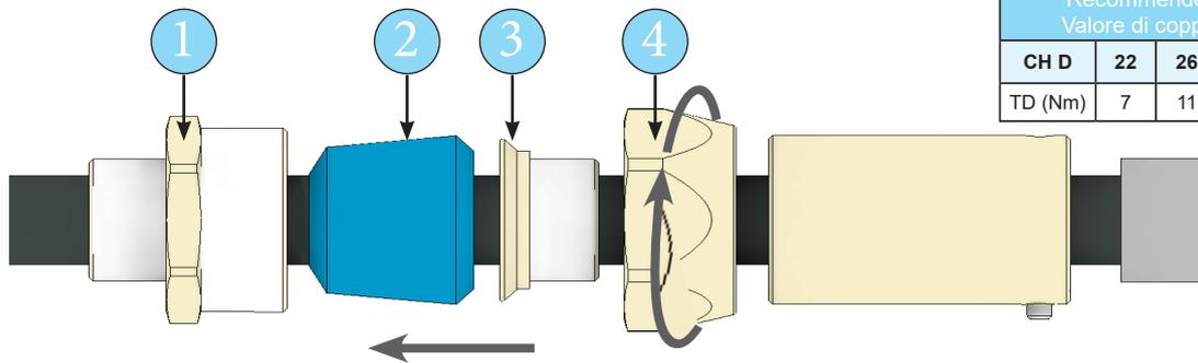
Recommended tightening torque value (TD)
